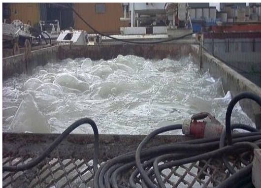
Agitation by an Air Compressor can Improve Mixing and Reduce Waste
