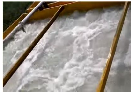
Agitation by an Air Compressor can Improve Mixing and Reduce Waste
