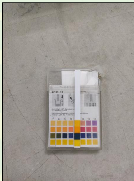
Photo 4: Reading test result: 10 using pH indicator strips (4 colours) for Fresh & Recycle Mixed
